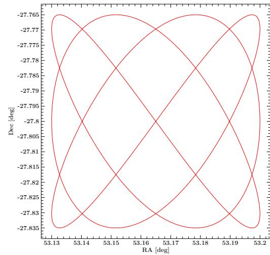
Dithering efficiently removes gaps between the chips.
