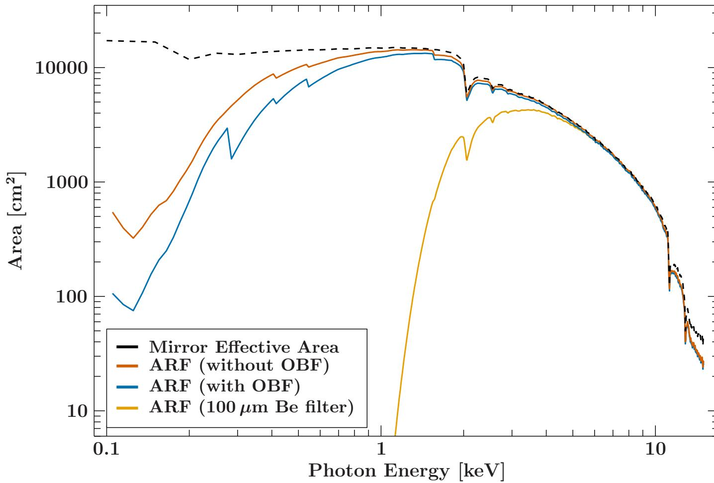
**Be filter**  $\Rightarrow$  removes photons below 2 keV
