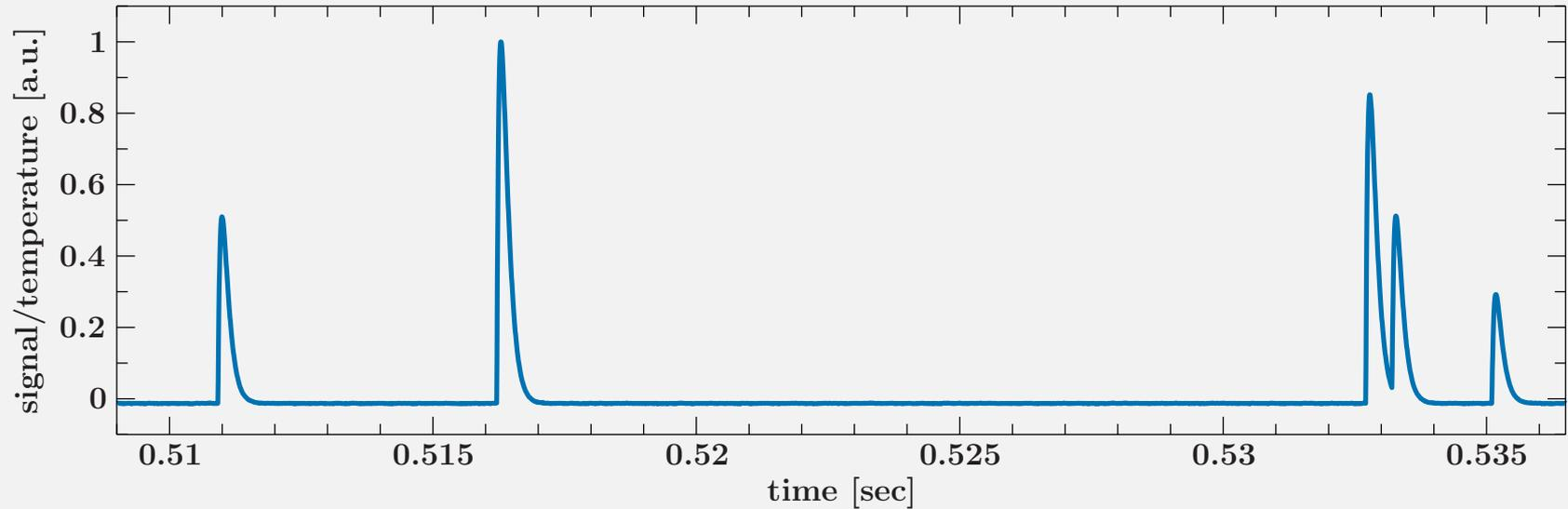
pulses with **smaller separation yield lower energy resolution**
