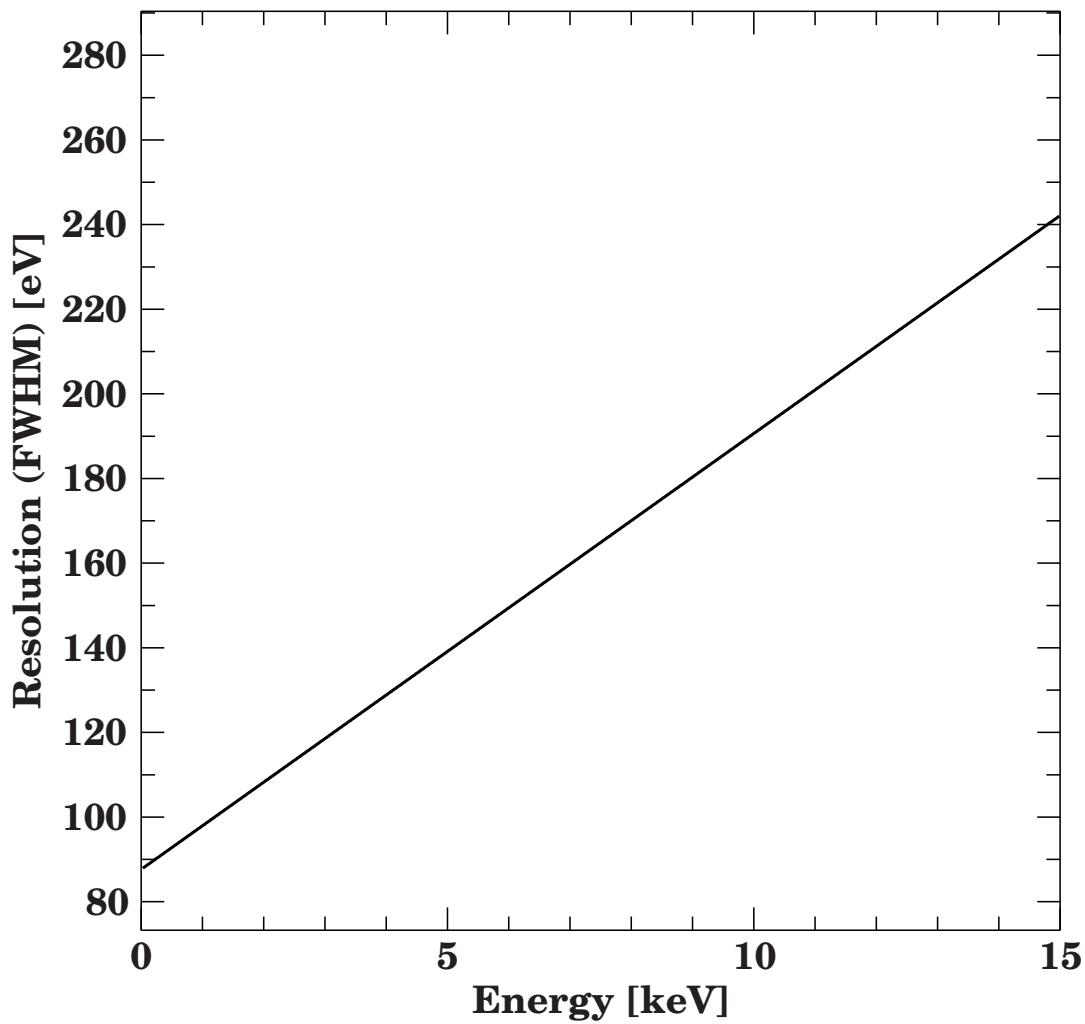
RMF composed of Gaussian with a width fit to lab measurements.
