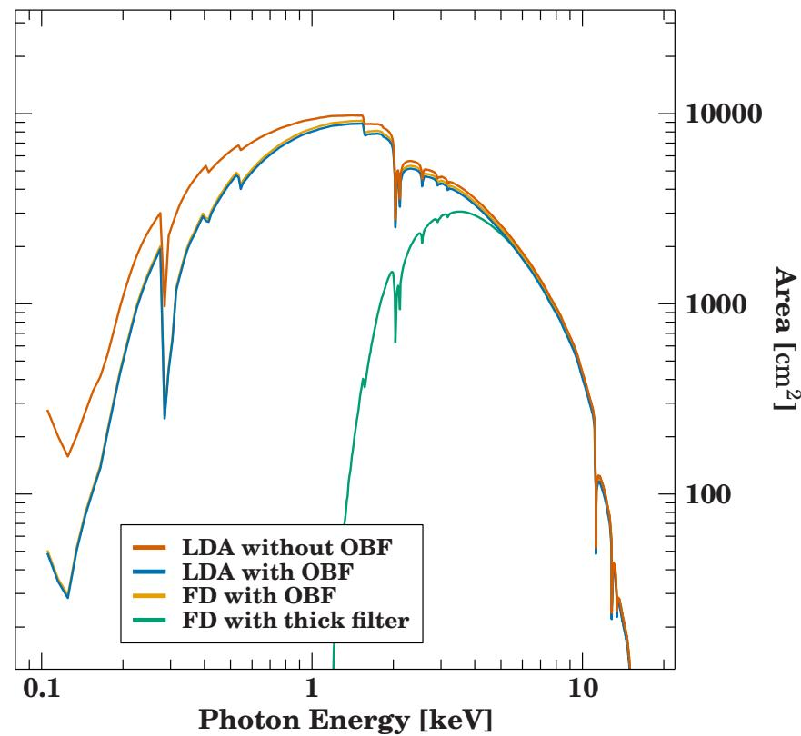
**Thick filter**  $\Rightarrow$  removes photons below 2 keV
