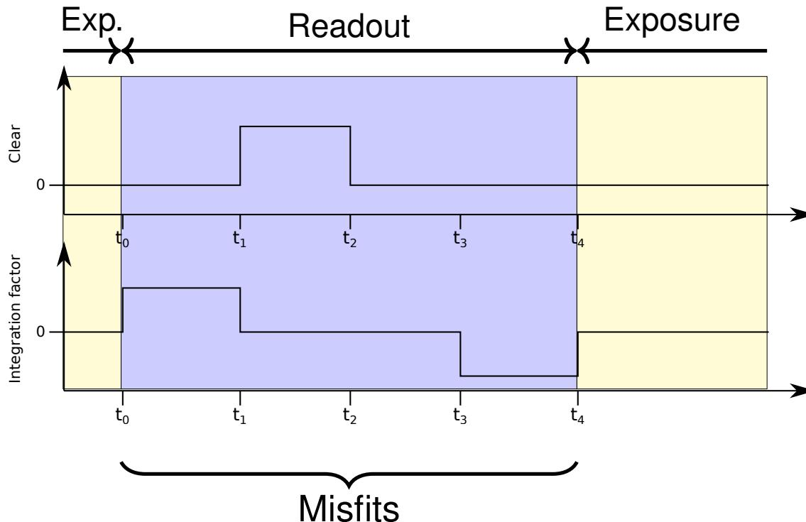
If photon hits during the read-out: measured charge is affected
