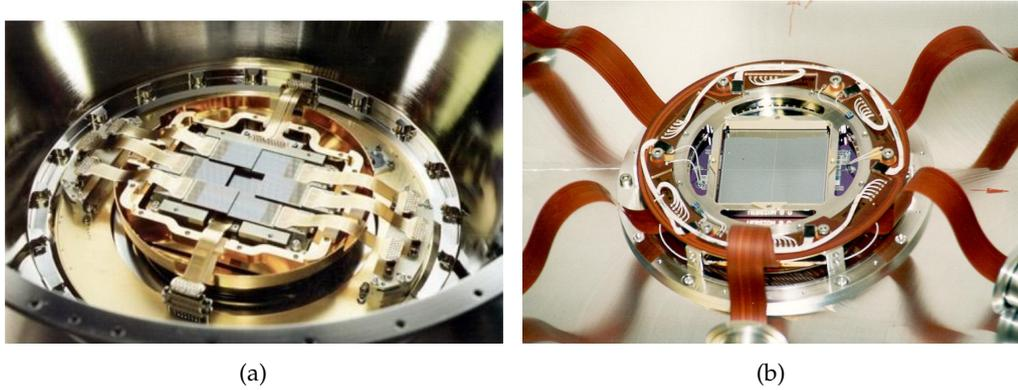
Figure 3.3: (a) EPIC MOS CCD array. Credit: Image courtesy of Leicester University, University of Birmingham, CEA Service d'Astrophysique Saclay and ESA. (b) EPIC pn CCD array. Credit: Image courtesy of MPI-semiconductor laboratory, MPE, Astronomisches Institut Tübingen, Germany and ESA.
