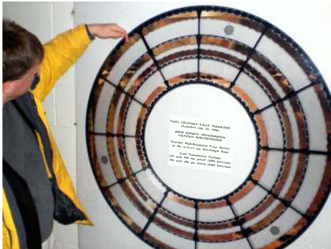
Figure 1.19: A true scale model of Chandra's High Energy Transmission Gratings (right), exhibited at MIT's Space Nanotechnology Laboratory, where the HETG were fabricated, with an X-ray astronomer (left) for size comparison. The two inner annuli contain 144 high-energy grating facets, whose gold transmission gratings have 5000 lines/mm, whereas the two outermost annuli consist of 192 medium-energy grating facets with 2500 lines/mm.
