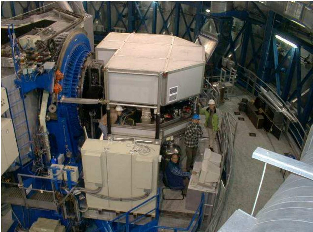
Figure 3.1: The Ultraviolet Visual Echelle Spectrograph (UVES) at the Nasmyth B focus of the UT2 telescope (Kueyen) of the VLT (picture taken from the UVES web-page <http://www.eso.org/instruments/uves>).
