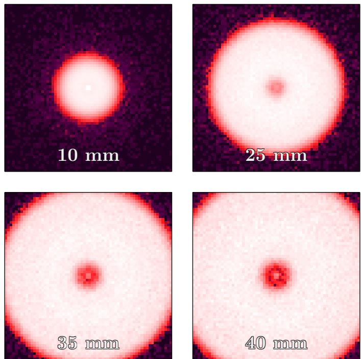
⇒ defocusing distributes photons over larger area (**35 mm is optimal**)
