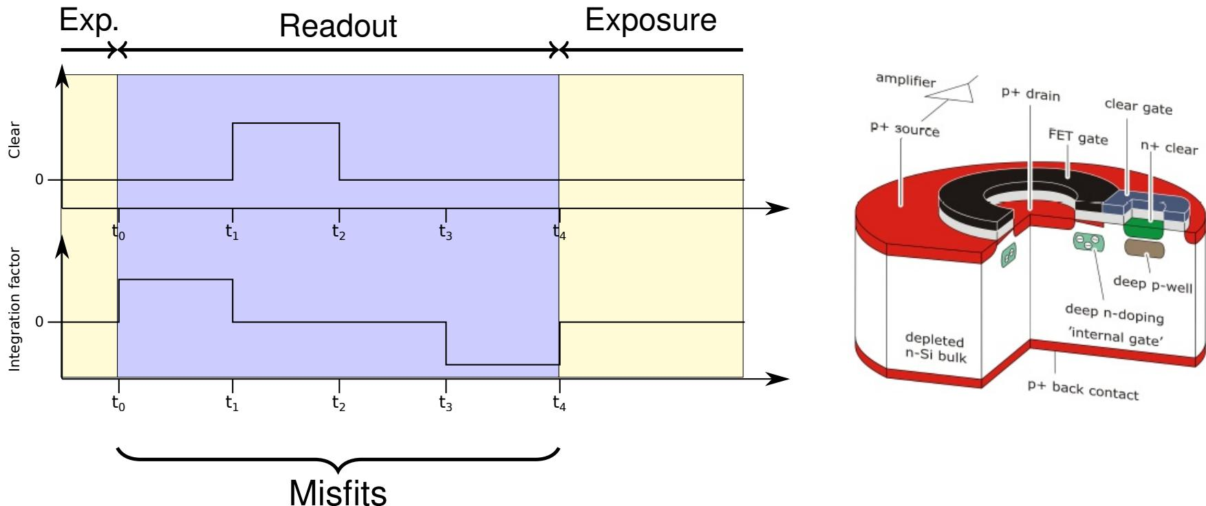
If photon hits during the read out: measured charge is affected
