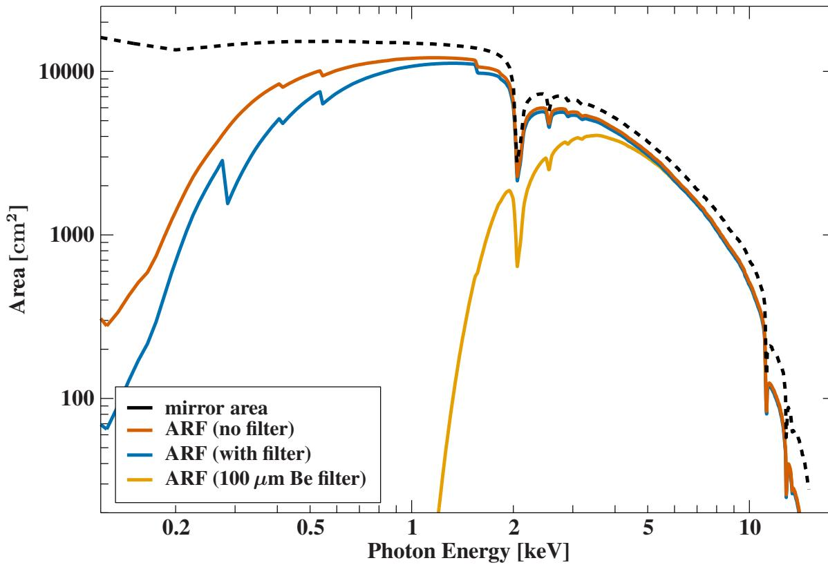
**thick Be filter** ⇒ removes photons below 2 keV
