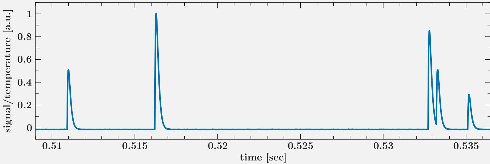
pulses with **smaller separation yield lower energy resolution**
