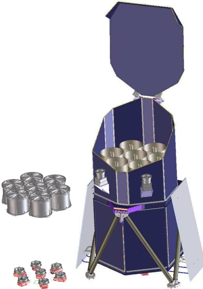
Figure 2.6: Configuration of eROSITA. Left: mirror systems and pn-CCD detectors surrounded by Cu proton shields. Right: final telescope configuration with Sun shield, mirror baffles, telescope tube, heat radiators etc. (Predehl, 2008b).
