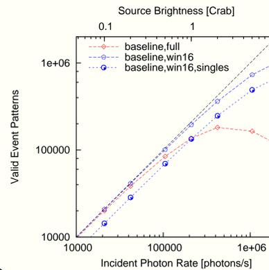
In the figure on the left-hand side the throughput of the HIFI instrument, i.e. the number of valid event patterns vs. the incident photon rate is displayed for simulated observations with different source brightness. The throughput is shown for the full frame and 16 × 16 window mode. For observations of very bright sources the instrument has to be operated in a window mode in order to cope with the high count rates resulting in pile-up problems.
