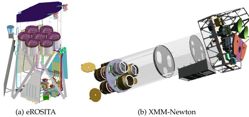
Figure 3.8: The X-ray telescopes named eROSITA (a) and XMM-Newton (b) are shown schematically, with their X-ray mirrors and detectors, in this Figure. From ESA: XMM-Newton SOC (2022) and Predehl et al. (2021).
