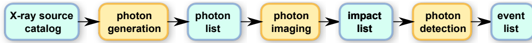
Figure 3.1: The basic layout of the standard SIXTE processing pipeline. In blue boxes, data products, either for in- and output or for optional intermediate files are shown. Yellow boxes depict the three main processing steps. Modified after Schmid (2012).
