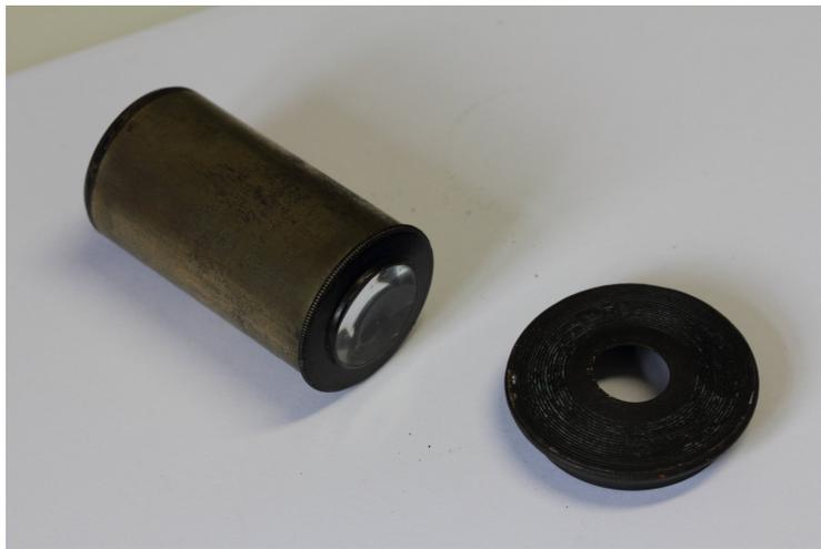
Figure A.4.: Components of eyepiece
