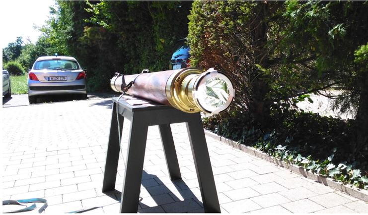
Figure A.22.: Modern sun filter on heliograph
