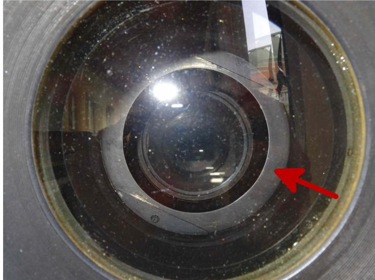
Figure 3.8.: Aperture stop in objective
