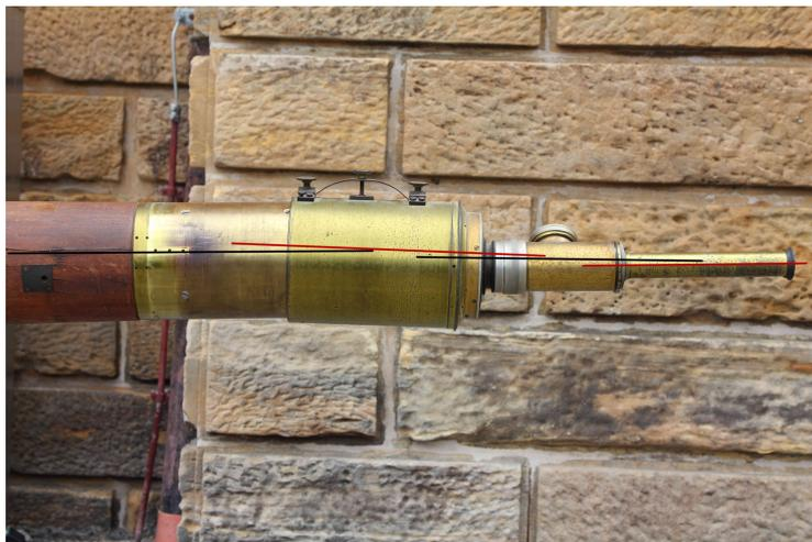
Figure 3.3.: Ocular with misaligned optical axes
