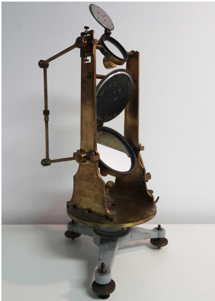
Figure A.19.: Lateral view of heliostat showing rods for parallel setting of mirrors
