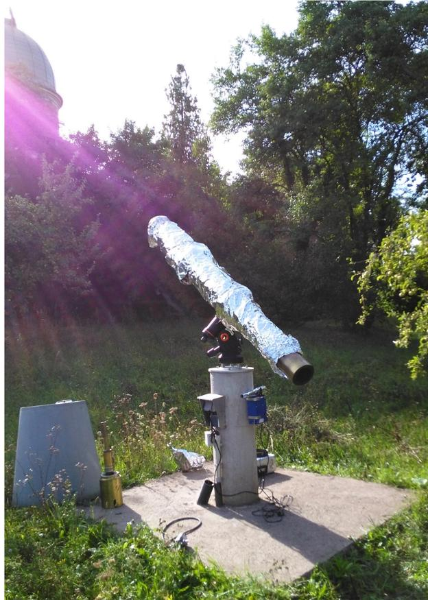
Figure A.16.: Refractor on modern mounting in Garden of Dr. Remeis Observatory, protected against heating up by tin foil
