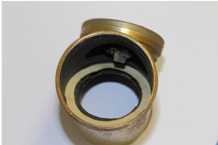
Figure A.8.: Centre component of eyepiece with prism and cardboard
