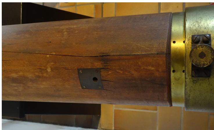
Figure A.21.: Fixing device for viewfinder on heliograph
