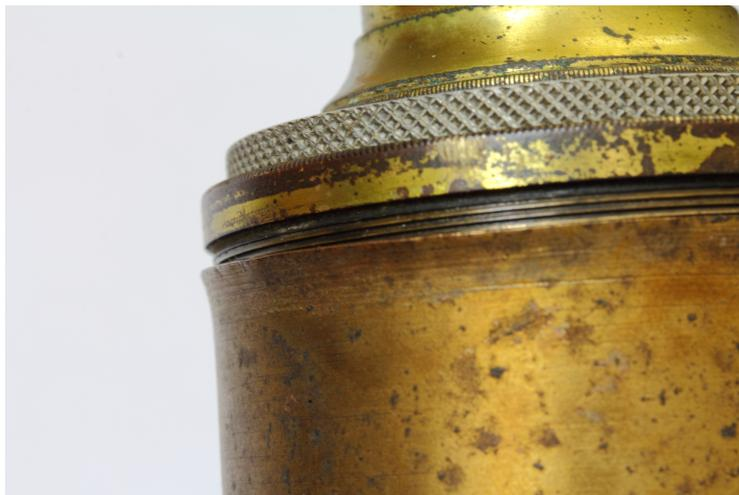
Figure A.1.: Damaged thread
