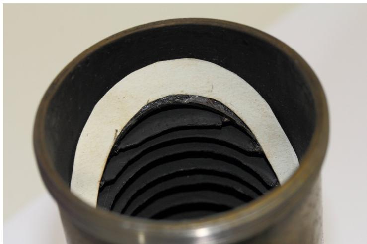
Figure A.7.: Cardboard to avoid reflection and scattering of light
