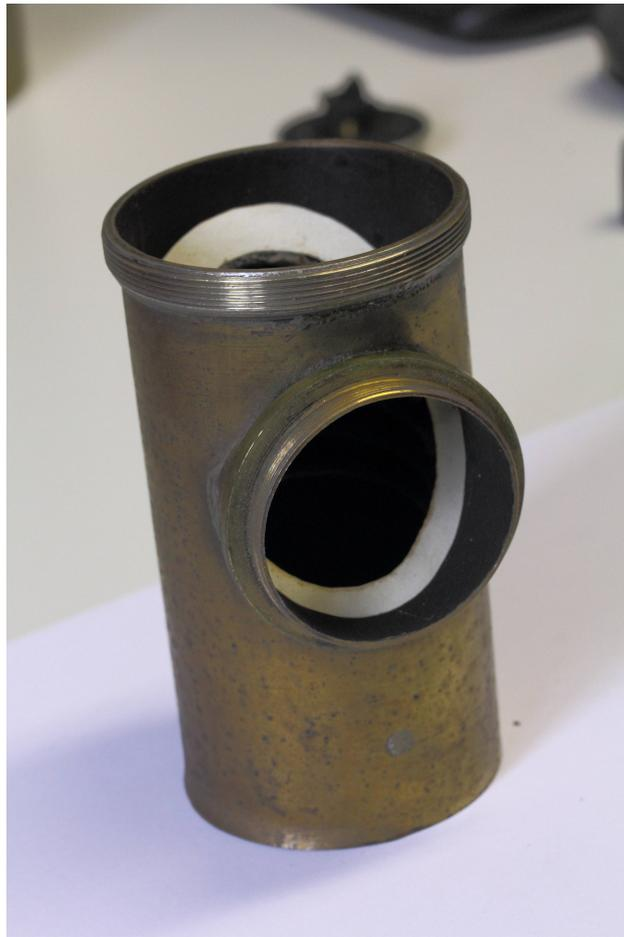
Figure A.6.: Centre component of eyepiece
