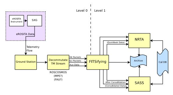
**Figure 2.7:** Illustration of the data flow starting on-board the eROSITA satellite transmitted to the ground station, processed and ending in the NRTA and SASS pipelines. Wilms et al. (2009)
