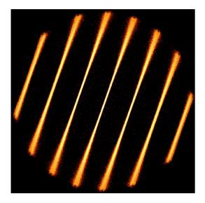
Figure 2.2: Simulated traces for one bright X-ray source caused by the continous slew of the eROSITA satellite (Schmid, 2012). The traces become wider towards the edges of the FoV caused be the degredation of the PSF for large off-axis angles.
