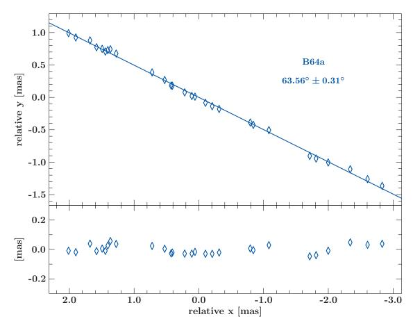
**Figure 4.24:** In the top panel the shifted x and y position of component B64a, with the mean of x and y centered at zero, is depicted. A two dimensional linear regression fit with the algorithm by Fasano & Vio (1988) is overlaid. The distances of the linear regression fit to the corresponding model component positions are shown in the lower panel.
