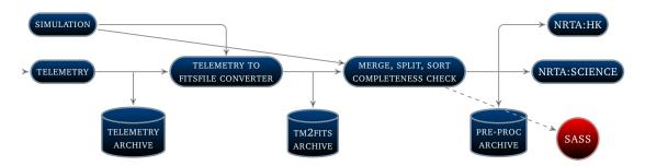
**Figure 2.9:** The pre-processing pipeline. The incoming telemetry data is converted into certain FITS files, which will be merged, split, sorted according to the requirements of the SASS or different parts of the NRTA.
