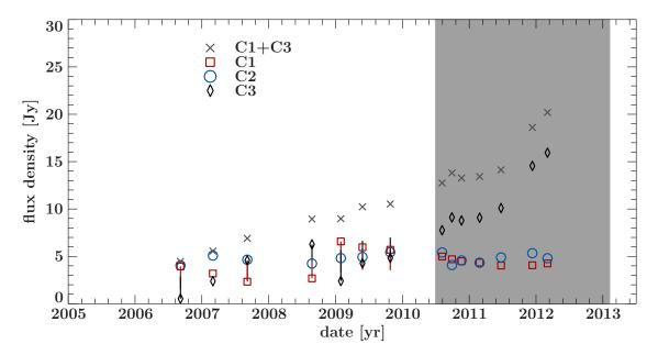
**Figure 5.10:** Light curve of the zones C1, C2, and C3 at 15.4 GHz. The flux density was derived by summing the flux density of all model components in each region. The uncertainties are based on the transition region marked, represented by the red lines in Fig. 5.6. The gray shaded area marks the same time range for which we obtained a light curve at 43 GHz.
