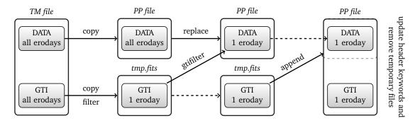
**Figure 2.12:** Processing of *TM file* if no *PP file* with the same specifications exists. The black boxes indicate a *FITS file*, while the shaded boxes the HDU extensions.
