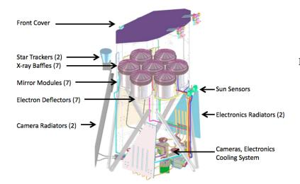
Figure 2.5: Schematic illustration of the eROSITA telescope structure with its various components. Predehl (2013)
