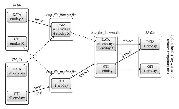
**Figure 2.13:** Processing of *TM file* if a *PP file* with the correct name already exists in the processing directory. The black boxes indicate a *FITS file* while the shaded boxes its HDU extensions.
