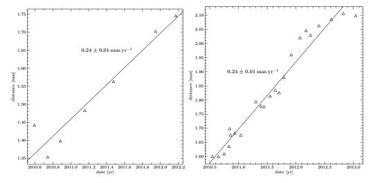
**Figure 5.8:** Distance of the flux weighted mean position of all components in zone C3 to the core component as a function of time at 15.4 GHz (*left*) and 43 GHz (*right*). A linear regression fit was applied to estimate the mean apparent motion of the region C3, which is  $0.24 \pm 0.01$  mas yr<sup>-1</sup> at both frequencies.
