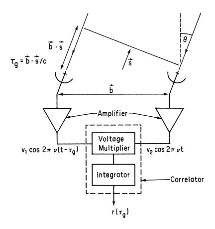
**Figure 3.2:** Two element interferometer with the baseline  $\vec{b}$  pointing in direction  $\vec{s}$ , and the expected geometric delay depending on  $\theta$ . Thompson (1999).
