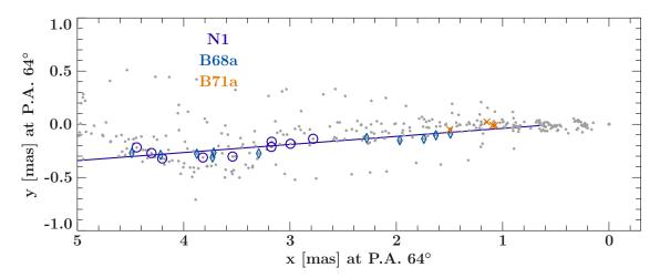
**Figure 4.14:** The positions of all model components rotated by 64° in gray. In indigo circles the model component positions of N1 are depicted and overlaid with a fitted linear trajectory. The predecessor candidates B68a and B71a are depicted in the same colors and symbols as in the previous figures i.e. Fig. 4.9.
