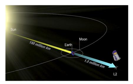
Figure 2.1: The eROSITA telescope will be the first X-ray telescope to view the X-ray sky in an orbit around Lagrange point  $L_2$ , which is a non-stable location of zero gravity. L2 is positioned on a straight line of the Sun and Earth connection, 1.5 million km behind the Earth not facing the Sun. (Credit: http://www.stsci.edu/jwst/overview/design/orbit)
