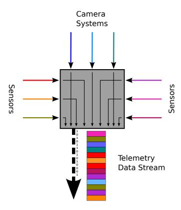
Figure 2.6: The composition of the telemetry data stream which will contain data packages from spacecraft sensors, the camera systems, state of instruments, etc. The composition of the telemetry data stream is not fixed and packages can be transmitted in any order.
