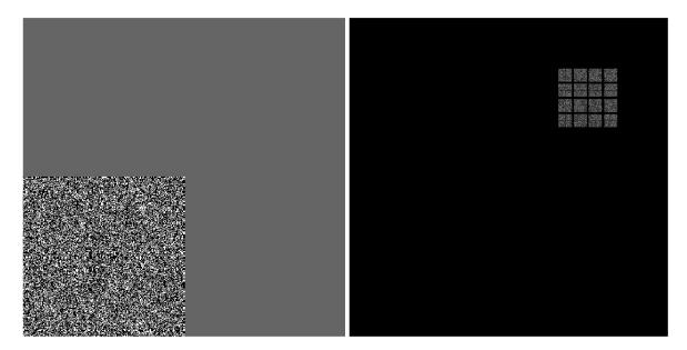
Figure 4.18.: Padding of the real arrays. The proportions fit those of the HXI and the gray area in the left image and the black area in the right one correspond to the padded zeros. The difference in color is due to the fact that the G array also comprises negative values and the color-coding is orientated at the lowest value as to equal the darkest.
