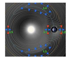
Figure 1.5: The 5 Lagrangian points. (from http://map.gsfc.nasa.gov/ m\_mm/ob\_techorbit1.html)
