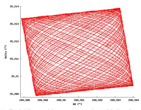
Figure 1.22: Chandra's Lissajous dither pattern: time-evolution of the focused target-position.
