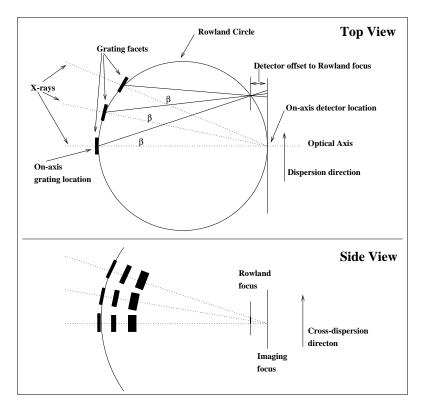
Figure 1.17: The Rowland geometry. (from http://cxc.harvard.edu/proposer/POG/html/HETG.html#tth\_fIg8.3)
