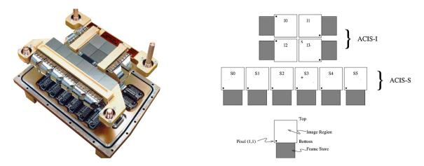
Figure 1.20: The ACIS CCD-chips: photography and sketch. Left: photography (from http://chandra.harvard.edu/about/science\_instruments.html), right: sketch (from http://chandra.harvard.edu/about/science\_instruments2.html).
