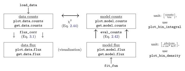
Figure 3.3: The main data structures for spectral analysis in ISIS and their interactions.
