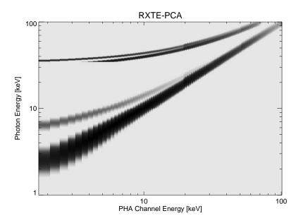
Figure 2.6: The response matrix of the xenon-gas Proportional Counter Array on RXTE.  $R(i, E) \equiv R(\text{channel, photon energy})$  (from Wilms, 1998, Fig. 4.4)
