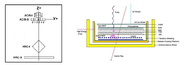
Figure 1.19: The Science Instrument Module SIM and the High Resolution Camera HRC. Left: SIM (from http://cxc.harvard.edu/proposer/POG/html/INTRO.html#tth\_sEc1.6), right: HRC (from http://chandra.harvard.edu/about/science\_instruments1.html).
