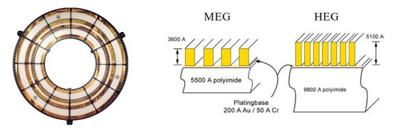
Figure 1.18: The High Energy Transmission Grating HETG.
