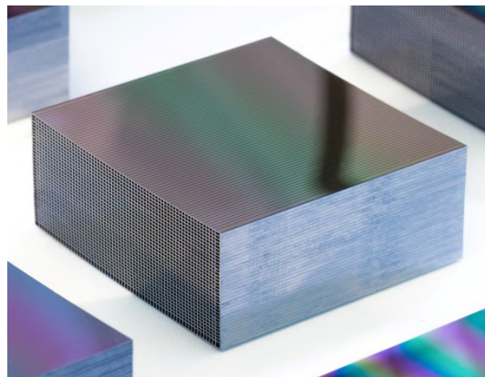
Figure 2.2: A SPO mirror stack with 35 layers of silicon plates. Each pore acts as a Wolter mirror to refract the X-rays back to the Focal Plane Module. Image from Collon et al. (2016).
