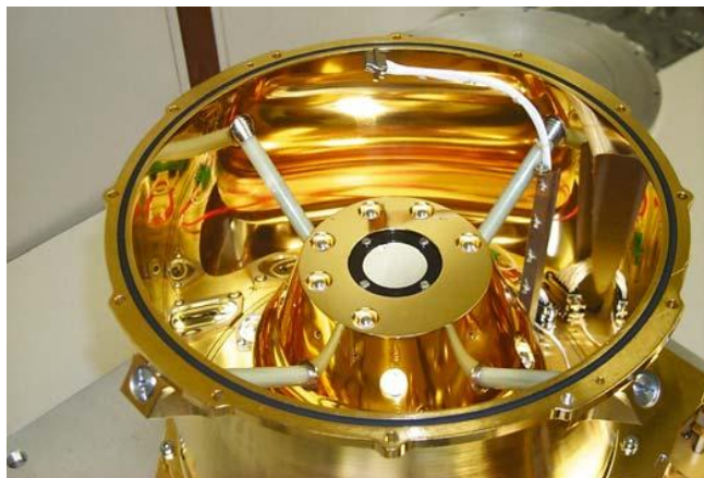
Figure 3.25.: XRT Blocking Filter(white circular filter) and Proton Shield in FPCA (Burrows et al., 2005)
