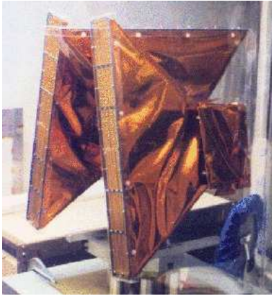
Figure 3.9.: Picture of the three SSCs of ASM, standing on their mutual rotation axis. The camera in the middle looks to the top and parallel to the rotation axis, while the cameras on the side look to the left of the picture.
