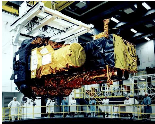
Figure 3.12.: Picture of INTEGRAL during testing at ESTEC. The coded masks are hidden behind golden foils. Note the persons in the back for size comparison. Picture credit: ESA
