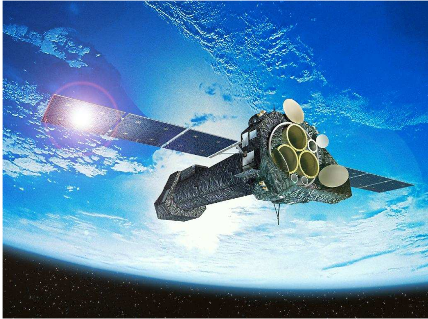
Figure 3.6.: Artistic view of XMM-Newton in orbit. Clearly visible are the three big X-ray telescopes to the right. The small telescope is the optical monitor. X-rays are focused and measured in the focal plane platform on the left. Picture credit: ESA.
