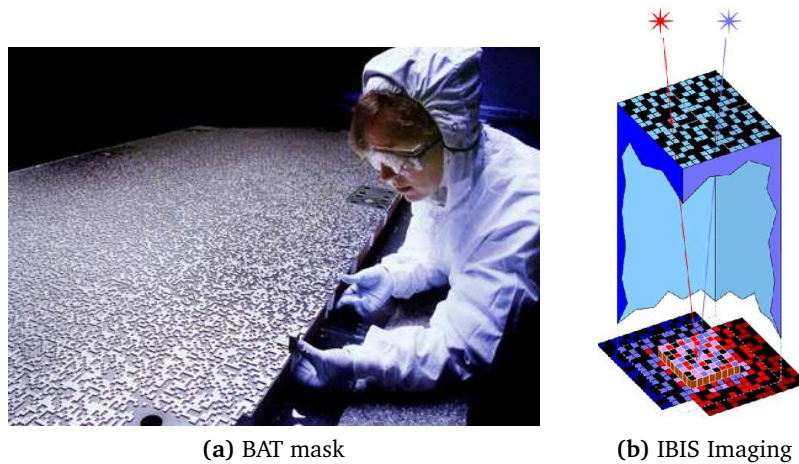
Figure 3.5.: (a) Photograph of Swift /BAT's coded mask during assembly. Picture credit: NASA (b) Sketch showing the different shadows cast by two different sources (red and blue star) through the mask of INTEGRAL /IBIS. Through the well-chosen pattern, the red and blue shadows are almost unique and the flux of each source can be reconstructed. Picture credit: ESA
