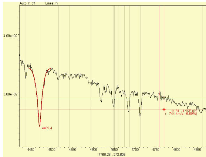
Figure 3.1: A screenshot of the plot window, showing a typical HeSDO spectrum from the SDSS database in black. Restwavelengths of a selection of spectral lines are marked by the vertical grey lines which highlight and print the species and ionisation stage on screen when under the mouse cursor. The red lines across the complete screen demonstrate the ruler function, where the distance of the current cursor position to a previous position is given in Ångström and flux (see red numbers at the lower right of the screenshot) as well as in velocity and relative flux (red numbers in parenthesis). A fit to the He I 4472 Å line is also shown (thick red line).
