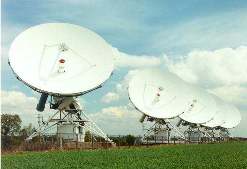
Figure 3.2: Compact configuration of the Ryle Telescope. 5 of its 8 elements, which can be moved on rail tracks, are grouped together. (Picture courtesy: www.mrao.cam.ac.uk/telescopes/ryle/ )
