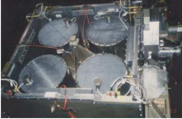
Figure 3.5: One of the two clusters of scintillation counters of HEXTE. (Picture from the NASA http://heasarc.gsfc.nasa.gov/docs/xte/learning_center/hexite.html )
