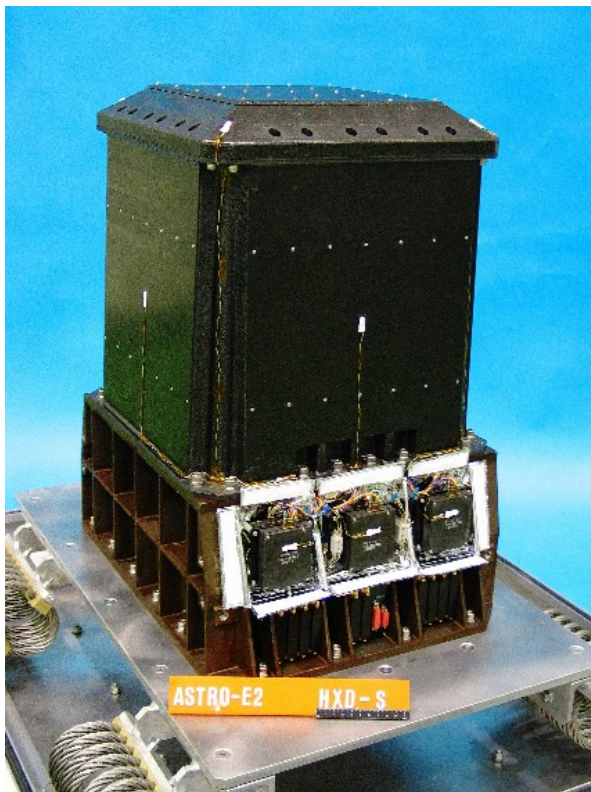
Figure 5.6: The hard X-ray detector. (Image courtesy NASA: http://heasarc.gsfc.nasa.gov/docs/suzaku/gallery/instruments/hxd.html )
