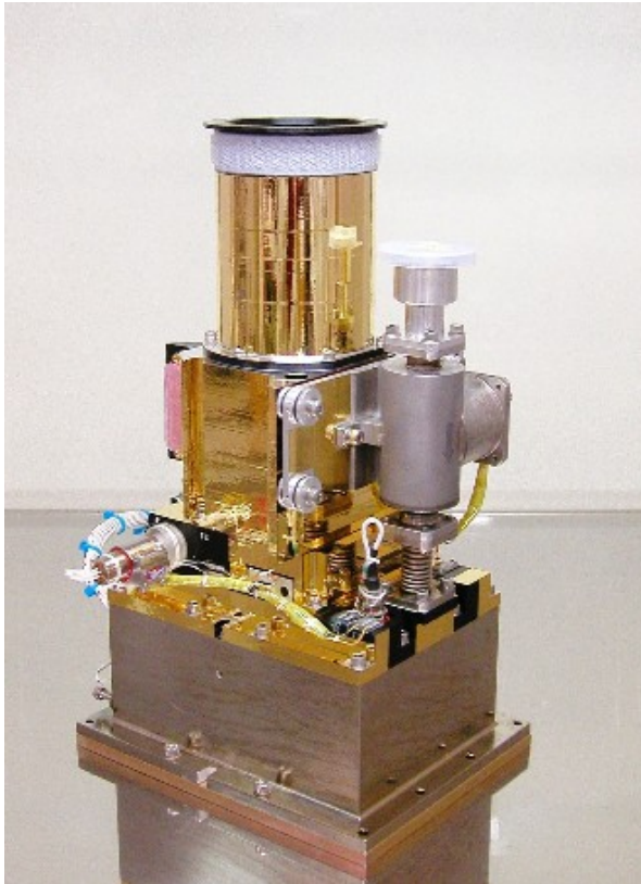
Figure 5.3: One of the four XIS detectors. (Image courtesy NASA: http://heasarc.gsfc.nasa.gov/docs/suzaku/gallery/instruments/xis.html )
